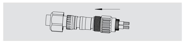
**Step 2:** Use Trox Driver T15 (recommended torque is 2~2.5 N.M) to terminate the 2 conductors in the corresponding contacts A, B in front plug assembly (item 1).
