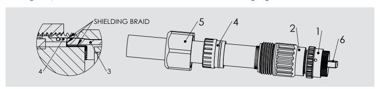
**Step 5:** Press the cable gland (item 4) down into a tightly seated position into the rear of the cable gland adapter.
