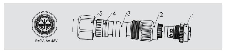
**Step 3:** Mate the dust cap onto the front plug and assemble the cable gland adapter (item 2) into position using an M30 spanner (recommended torque is 6~8 NM).
