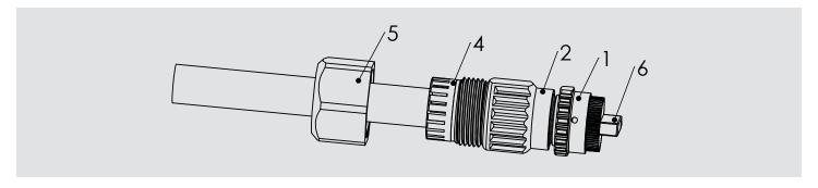
**Step 6:** Use the adapter as a fixture, hold on the adapter (item 2), fix the cable gland nut (item 5) in position with a 35mm spanner (recommended torque is 8~12 NM).
