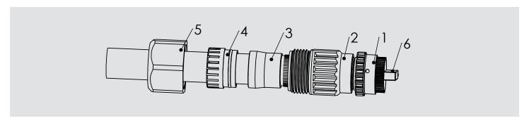
**Step 4:** Slide the shielding ring into the adapter along the cable until immovable, then tear off the tape with the shielding braid, at last fold the braid around the end of surface for the shielding ring.
