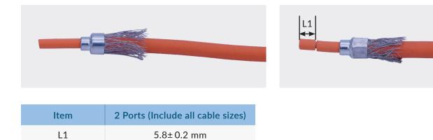
**Step 4:** Stripping the jacket and cut off the exposed shielding wire of cable, crimping the terminal by right crimping tool.
