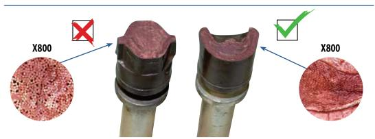
The W-crimping (on the right), allows a gas-tight crimp, avoiding oxidation. The strands are uniformly distorted and squeezed together, granting the best conductivity.
