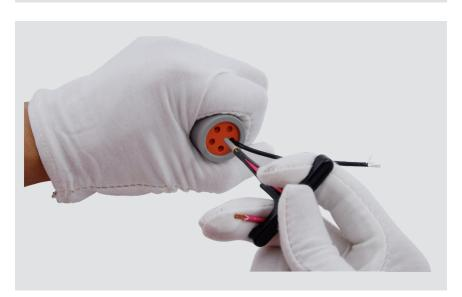
**NOTE:** The tool and wire should be fixed together and not loose when pulling out the terminal.
