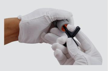
**Step 6:** Continue to press on the removal tool until it is unable to insert any longer. At this point the tool has fully unseated the terminal from the insert. Now pull on the tool and wire together to remove the terminal.
