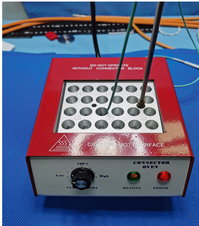
Figure 4-3 (position terminus into curing oven)
